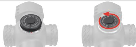
Once the scope has been sighted in, the elevation and windage adjustments can be set to zero.
