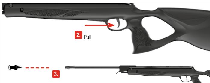
Never pull the trigger when the rifle is cocked and the barrel is broken open (exception - decocking, see above). The barrel would jump up, bend and possibly cause injuries. The piston would hit the cocking rod, possibly breaking. The stock could also crack or break. **This would void the warranty.**
