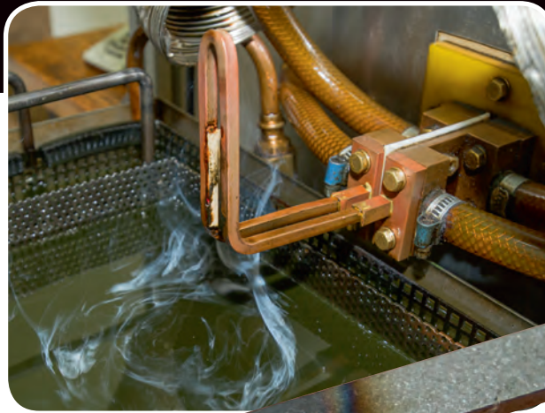
Group left: This part-tempering process for a trigger sear is carried out skilled technicians
