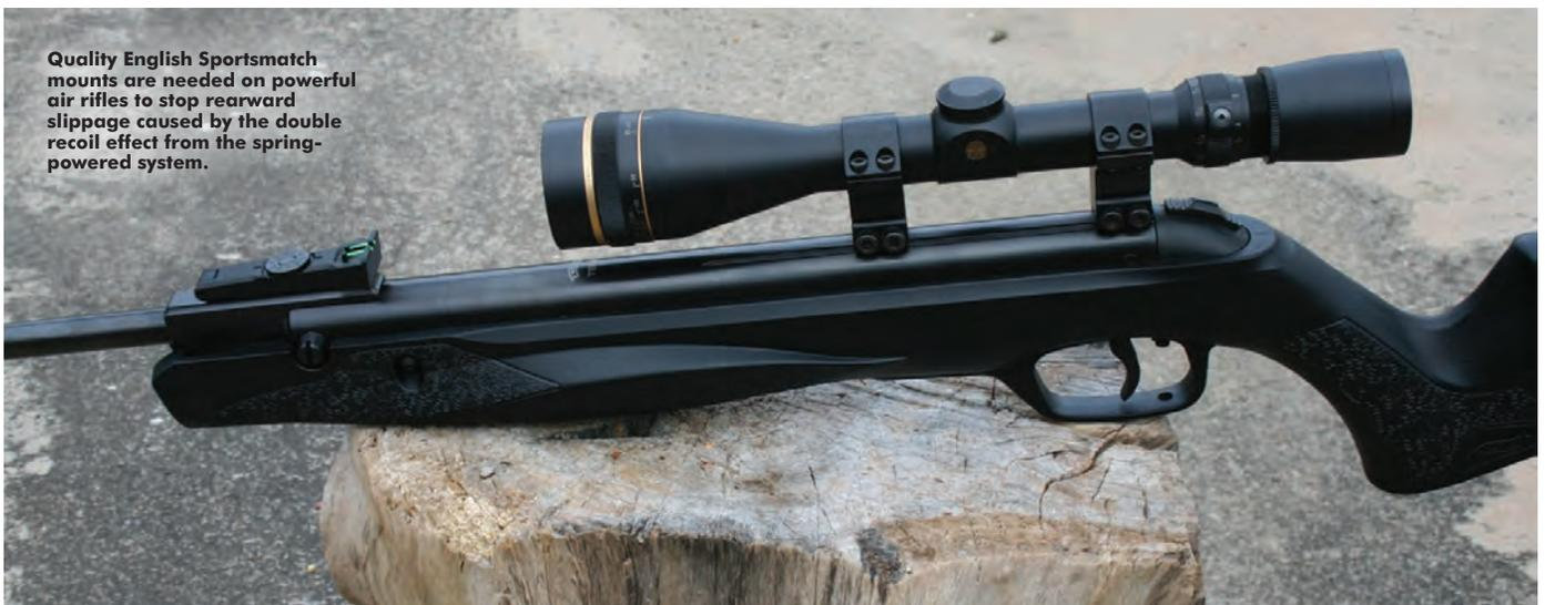
Quality English Sportsmatch mounts are needed on powerful air rifles to stop rearward slippage caused by the double recoil effect from the spring-powered system.
